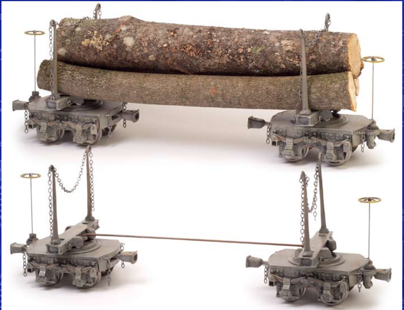
Photo Below: Pechot Bogies with log bolsters and empty showing spacer bar.
